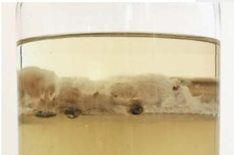
*Pictured above: Diesel Bug forming between water and diesel*
